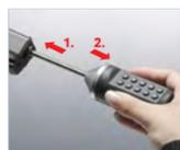
Release the locking mechanism by pressing the control unit slightly against the locking element, then pull the locking element carefully out of the barrel. If the locking element cannot be released, repeat the whole procedure.
